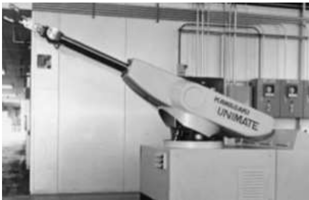
Figure (1) shows the first robotic machine (uinmate), which is a robotic arm connected to a giant steel cylinder that casts metal into molds, welds car bodies and lifts cars weighing 500 pounds.
