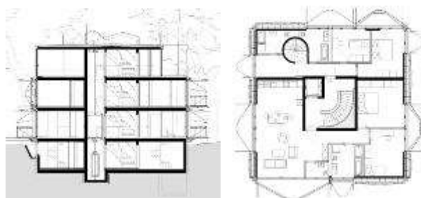
Figure“15”: Section reveals a composition of three floors above ground and one basement level. - First plan.
